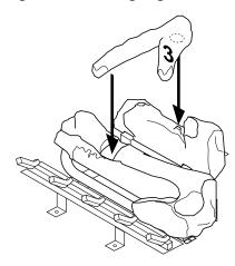
Figure 45 - Installing Log No. 3
